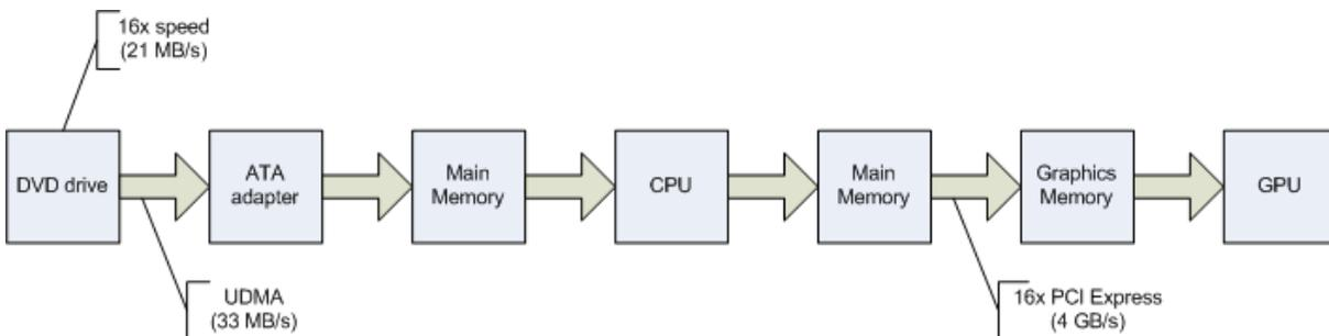
In this particular pipeline a 16x speed DVD drive is used. Ignoring seek times, the peak outer edge throughput of a 16x speed DVD drive is 21 MB per second. This is equivalent to a little over 7 MegaTexels per second (MT/s) of uncompressed RGB data. However, this throughput is never achieved in practice where a certain amount of seeking is unavoidable and bandwidth may
