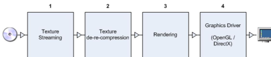
Current graphics drivers either cannot be orchestrated from multiple threads, or need to be synchronized first. As such, there is only one thread talking to the graphics driver, which is the renderer. The driver itself is typically also threaded
