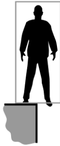
Fig. 4. A robot partly standing over a ledge while the bounding box rests upon the edge.
